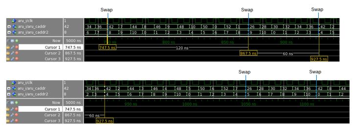
Figure 4.6: ARU Dynamic routing, swap mechanism: One port, DYN\_CLK\_WAIT = 0, DYN\_CLK\_WAIT 1
