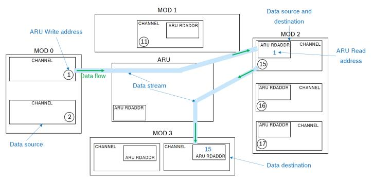
Figure 2.2: Example for ARU Routing mechanism
