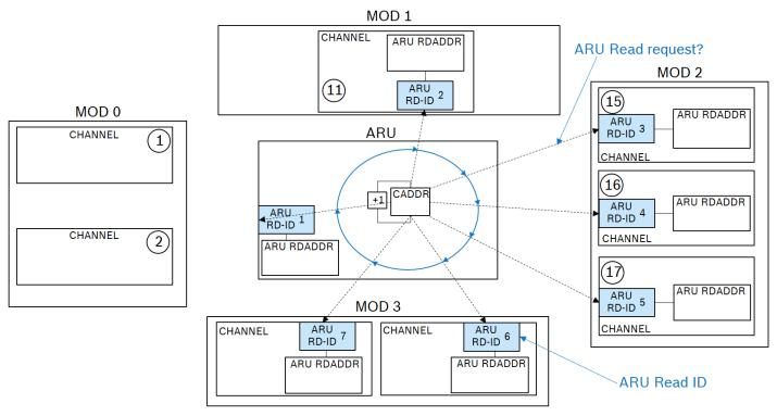
Figure 3.1: ARU Routing scheme
