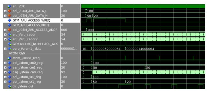
Figure 5.2: Default ARU access via CPU, CPU acts as ARU Write channel
