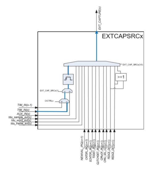
Fig. 6: TIM EXTCAPSRC subunit to generate TIM\_EXT\_CAPTURE(x) signal.
