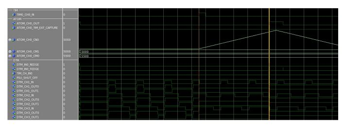
Fig. 8: Simulation result for use case 1, DTM outputs at defined state after shut-off time expired.
