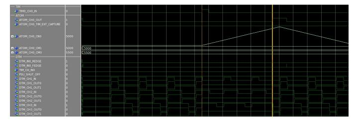
Fig. 10: Simulation result for use case 2, DTM outputs return to DTM\_IN after shut-off time expired.
