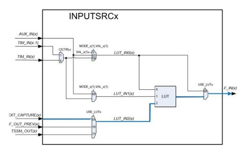
Fig. 7: TIM INPUTSRC subunit and the routing of the EXT\_CAPTURE(x) signal to TIM output signal.
