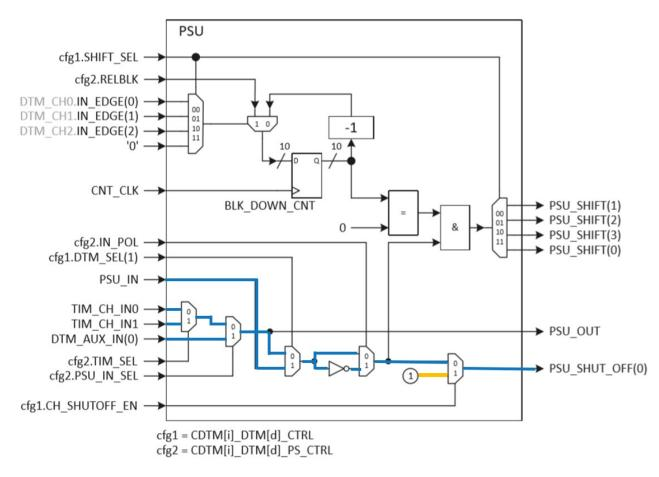
Fig. 2: Sources and routing of shut-off signal.
