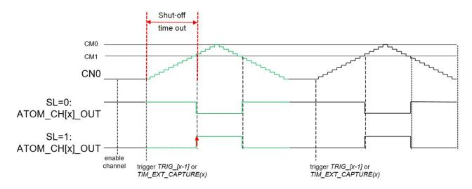
Fig. 5: PWM Output in one-shot counting up-down mode triggered by TRIG\_[x-1] or TIM\_EXT\_CAPTURE(x).
