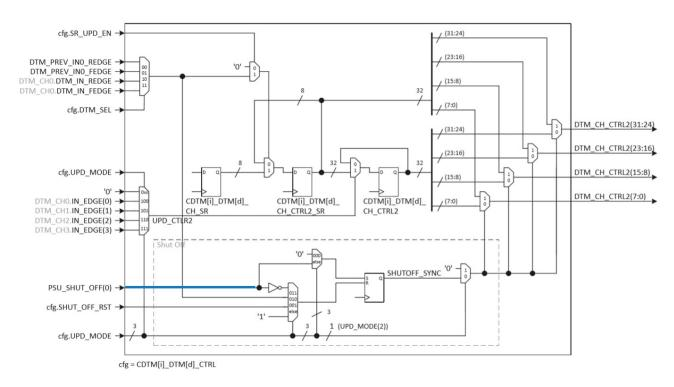
Fig. 3: Synchronous update mechanism of register DTM\_CH\_CTRL2.
