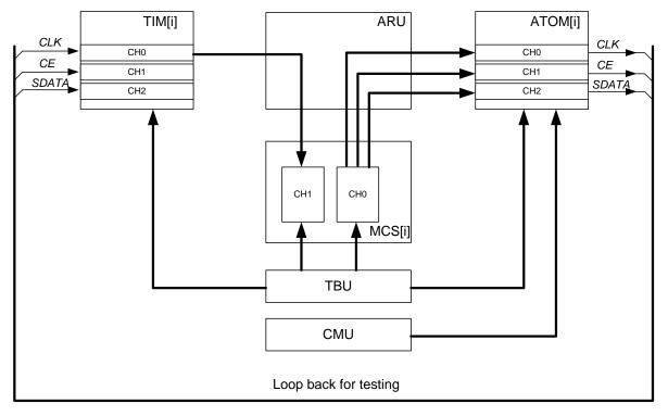
Figure 1.2: Application of the SPI functionality on the GTM device.
