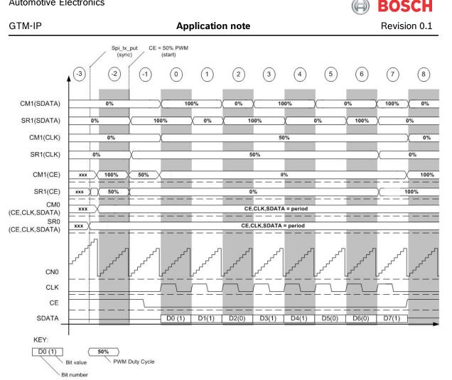
Figure 2.1: Timing diagram with additional ATOM Registers
