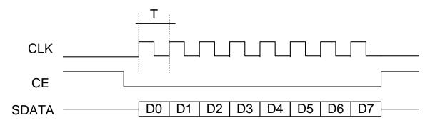
Figure 1.1: Timing diagram of SPI protocol.
